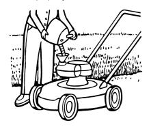
If you add gasoline to an engine that is running or hot, the result can be an explosion. Before you add gasoline, stop the engine and let the engine cool for several minutes. Remove dry grass and other debris from the mower. Keep the mower clean to improve the performance, help the engine and transmission run cooler, extend the life of moving parts, and decrease the danger of a fire.
